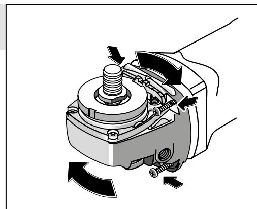
**2. Установка защитного кожуха**
